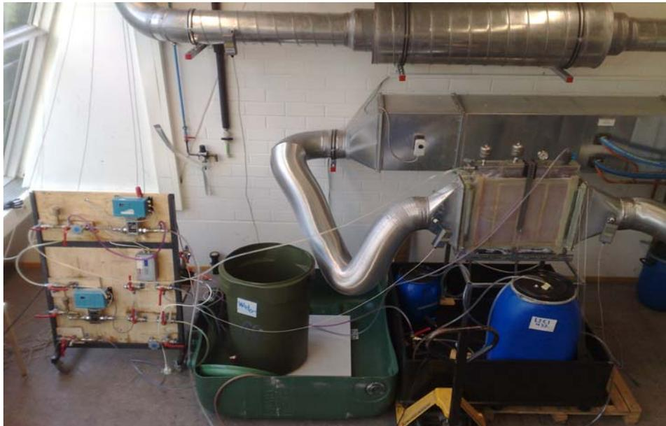
Fig. 2. Liquid desiccant absorber, connected to the air and hydraulic test rigs in the pilot plant stage in the laboratories of Kassel University (August 2009).
