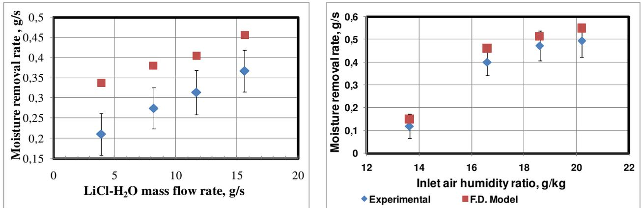
Fig. 5: the moisture removal rate as a function of desiccant flow rate and air inlet humidity ratio for the dehumidification experiments.
