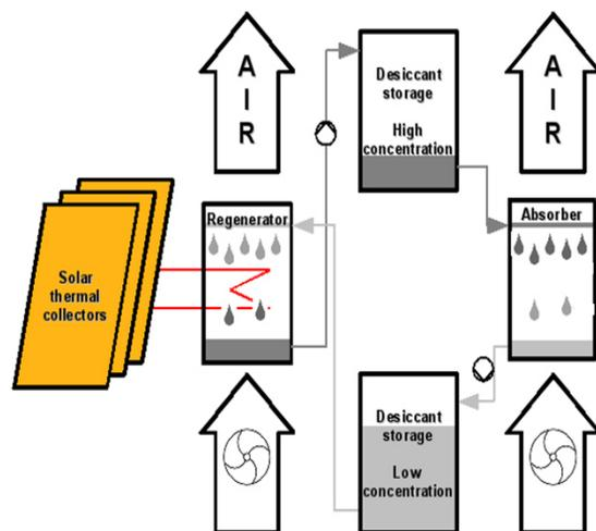
Fig. 1: Schematic of the liquid desiccant system.
