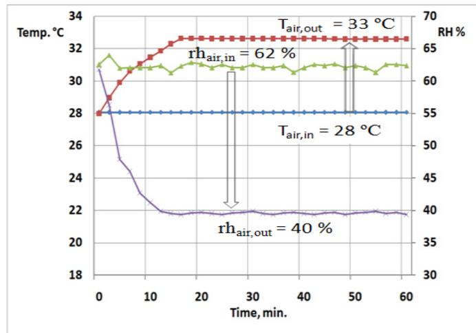
Fig. 4: Example measurement: Dehumidification in a small laboratory prototype.
