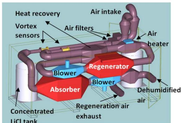
Schematic diagram of the exp. setup
