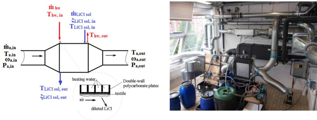
Fig. 2 Schematic diagram of the experimental setup, pilot plant stage
