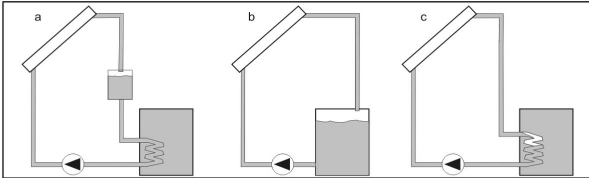
Picture 1 - Drainback systems in accordance to the location of the volume of the drained heat carrier: a) drainback vessel, b) heat storage as drainback vessel, c) oversized heat exchanger
