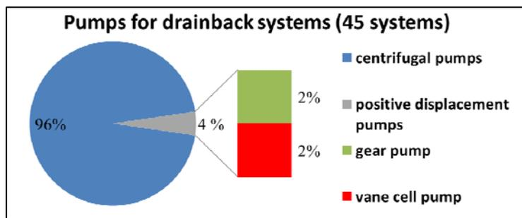
Picture 4 – Pump types used for drainback systems
