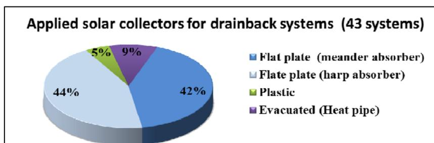
Picture 2 – Applied collectors types for drainback systems from different manufacturers
