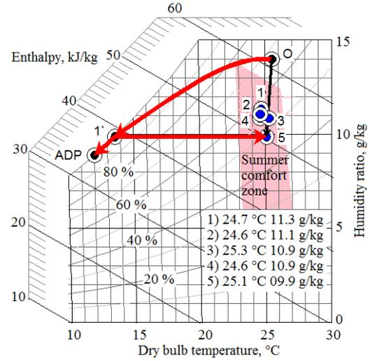
**Fig. 4. Experimental results of supply air conditions (dehumidified air) and schematic dehumidification cycle in the psychrometric chart for an internally cooled and a conventional vapor compression processes.**
