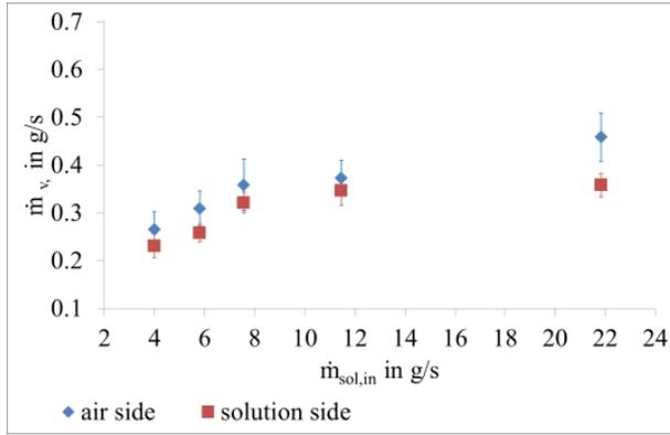
**Fig. 3: Experimental results.** Water vapor mass flow rate calculated from measured temperatures and humidity at the air side (diamonds) and from measured temperatures and density at the solution side (squares) over the solution mass flow rate.
