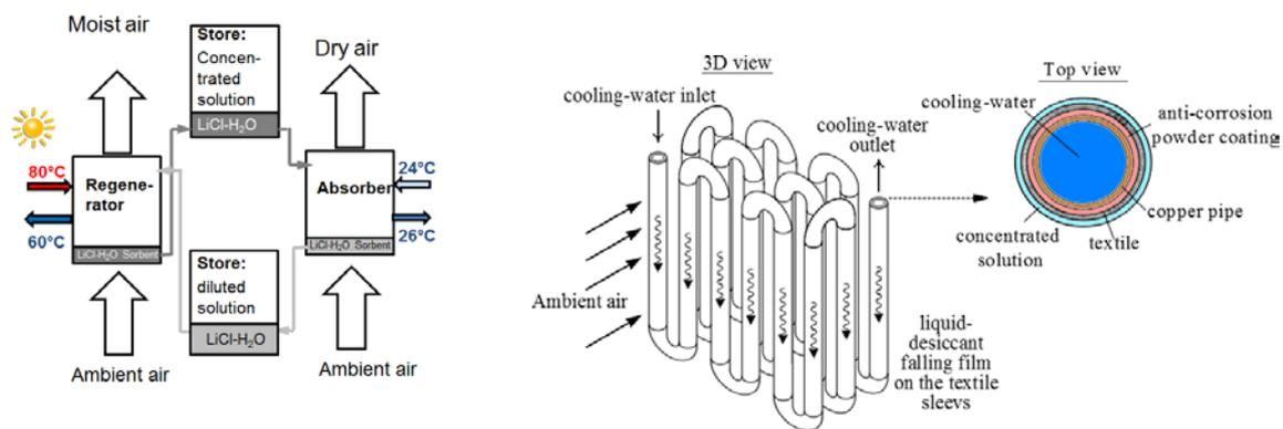
Fig. 1: Liquid desiccant air conditioning system. Fig. 2: Tube-bundle dehumidifier (left), cross section of the tubes (right).
