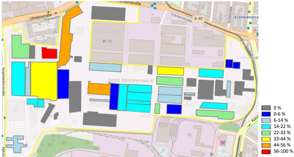
Figure 2: Standardised specific annual heat consumption of the different buildings in an automotive manufacturing plant (floor space)
