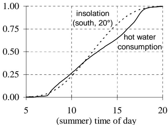
**Fig.3: Mean sums over the entire measurement period of the insolation on an inclined surface and the energy of hot water consumption, normalized. Despite appreciable deviations of single values from the mean value the two quantities correspond well. The hot water consumption is nearly constant over the day with a demand-peak in the late afternoon.**
