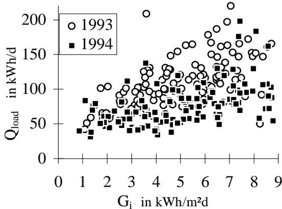
Fig.1: Daily sums of the supplied energy for hot water consumption  $Q_{load}$  versus the insolation on a tilted surface  $G_i$  (oriented to south, 20° inclination), measured at the public outdoor swimming-pool in Marburg (Germany)
