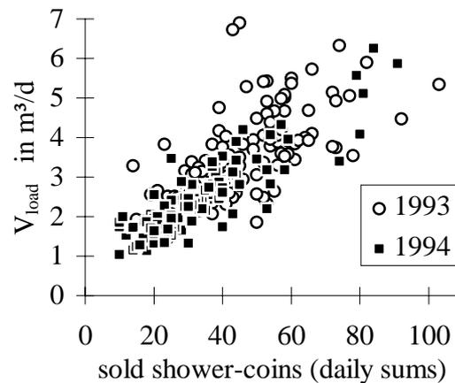
**Fig.4: Daily sums of the supplied hot water volume (40°C) versus the sold shower-coins. Obviously the number of shower-coins can lead to a useful estimation of the hot water demand, if no other measured data are available.**
