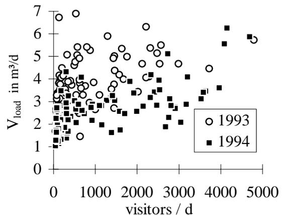
Fig.2: Daily sums of the supplied hot water volume  $V_{load}$  (40°C) versus the number of visitors. Surprisingly, both quantities are nearly uncorrelated.
