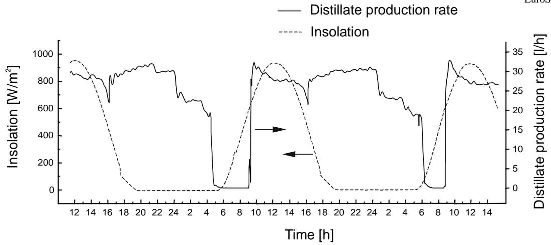
Fig. 4: Distillate production rate and insolation of July 21 and 22, 1997
