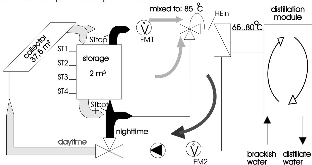
Figure 3: System scheme of the desalination plant installed in Sfax
