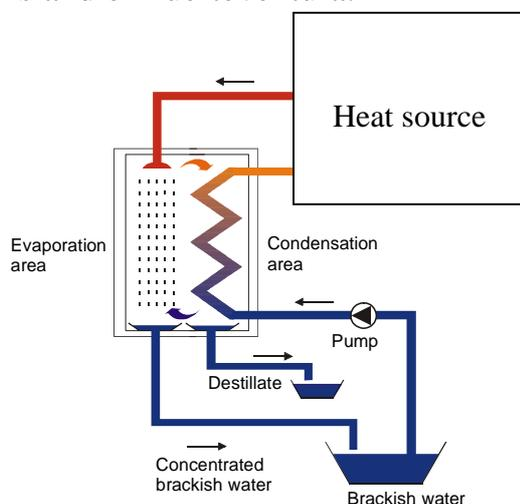
Figure 1: Illustration of the multi-effect-distillation without storage implementation
