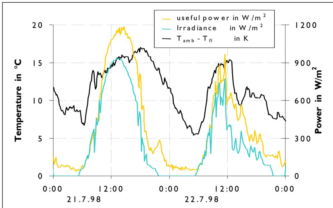
Figure 3. Measured quantities of  $T_{amb} - T_{fl}$ , power and irradiance.
