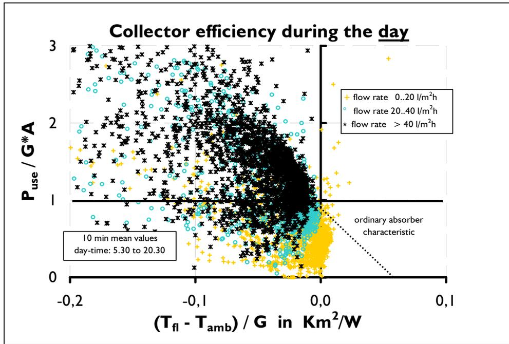
Figure 4. Measured 10 min mean values of the collector efficiency, which increase with increasing flow rate. The collector efficiency is nearly always > 1 at high flow rates. (June to August 1998)
