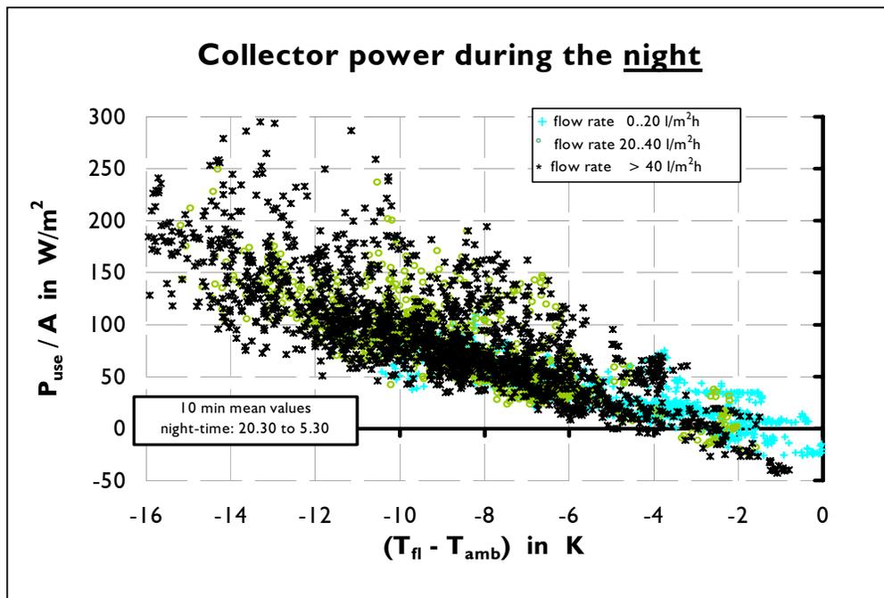
Figure 5. Measured 10 min mean values of the collector power. Even at night remarkable heat gains, nearly independent of the flow rate, were measured. (June to August 1998)
