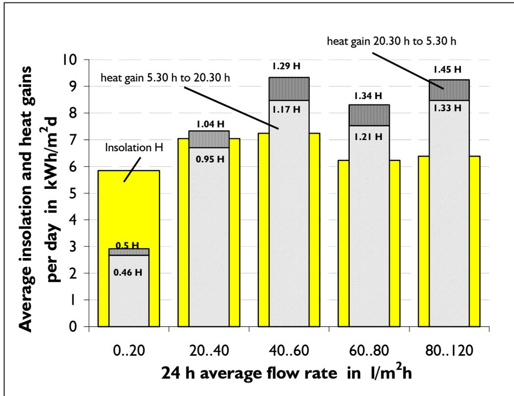
Figure 6. Average values of daily insulations and heat gains. The best results could be observed at high flow rates
