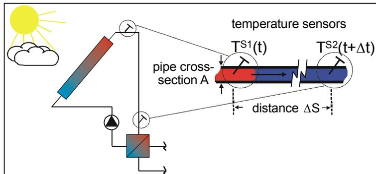
Figure 1: Schematic principle of the flow rate measurement on the basis of analyzing temperature steps
