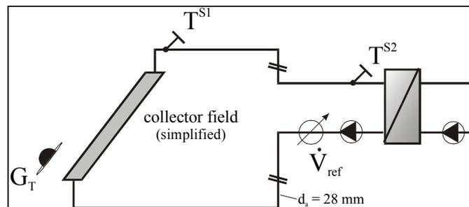
**Figure 3: Sketch of the collector circuit with the relevant measuring points.**
