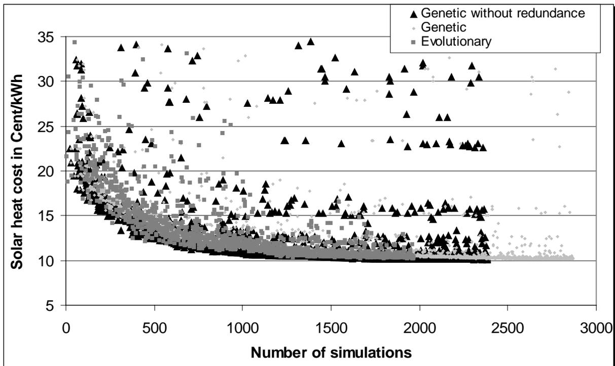
Figure 5: Optimization of System B, carried out with a Genetic Algorithm and with an Evolutionary Strategy. The third curve represents the development of the Genetic Algorithm without the redundant simulations.
