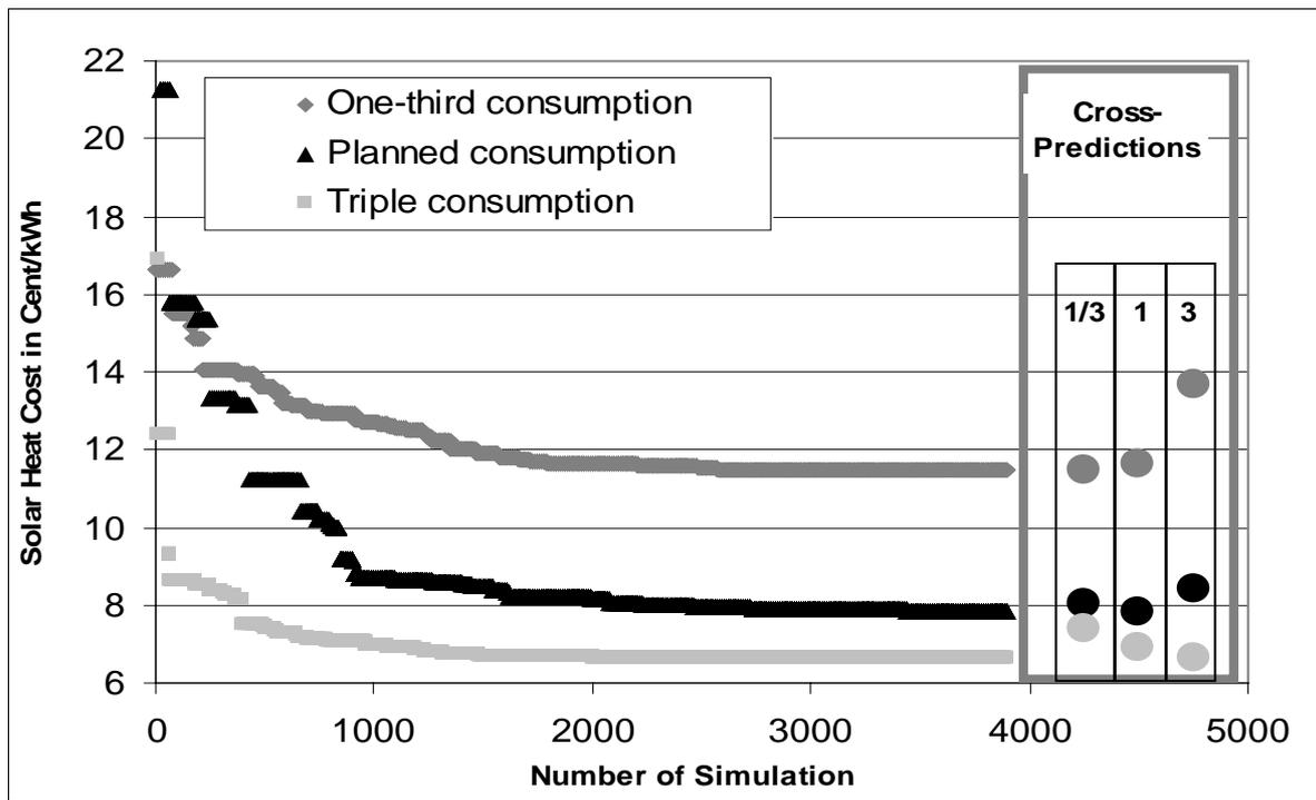
Figure 4: Dependency of the optimization result on the hot water consumption at System A carried out with a Genetic Algorithm. The dots in the rectangle on the right hand side of the diagram represent the cross-predictions, which are carried out with the parameter vectors determined from the optimization with the other amounts of consumption.
