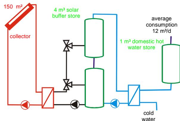
**Figure 2: Design of the smaller SHW-system ("System B",  $f_{sol} \approx 28\%$ ).** A discharge of the solar buffer store takes place only during the tapping of hot water.
