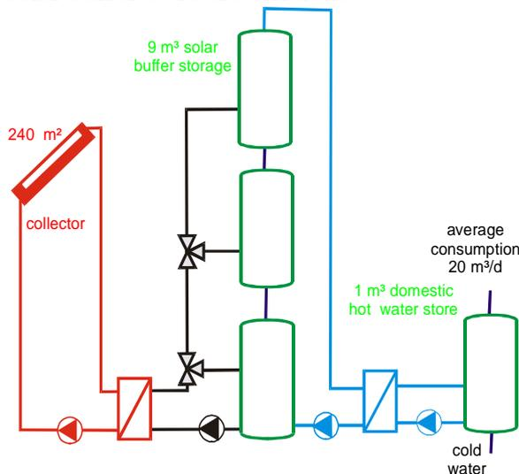
**Figure 1: Design of the larger SHW-system ("System A",  $f_{sol} \approx 30\%$ ).** A discharge of the solar buffer store takes place if the temperature level in the DHW store is below the temperature in the upper solar buffer store.
