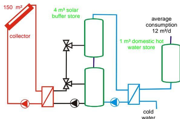
Figure 1: Design of the SHW-system ( $f_{\text{sol}} \approx 28\%$ ).
