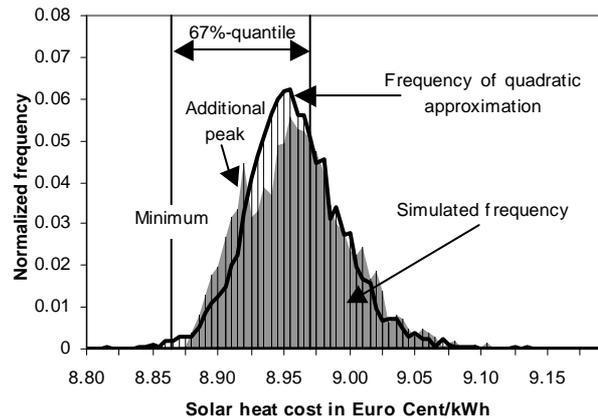
Figure 5: Normalized frequency of the solar heat cost of the different system configurations obtained by 3000 simulations generated with MCA. The grey distribution represents the simulated values, the distribution with the black curve shows the same for quadratic approximations, cf. text.
