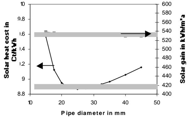
Figure 3: Sensitivity of solar heat cost and solar gain on the pipe diameter, determined with DSA. The grey ranges represent deviations of the objective function and the solar gain respectively of less than 1 %.
