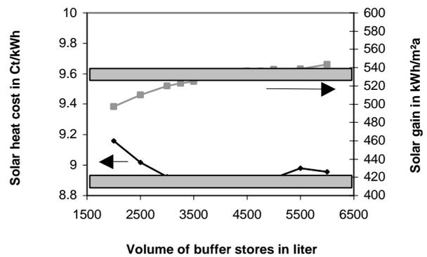
Figure 4: Sensitivity of solar heat cost and solar gain on the buffer store volume, determined with DSA. Again, the grey ranges represent deviations of the objective function and the solar gain respectively of less than 1 %.
