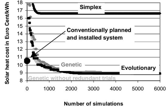
Figure 2: Development of the simulated solar heat cost for the investigated system depending on the number of required simulations. The optimizations have been carried out for three different algorithms.
