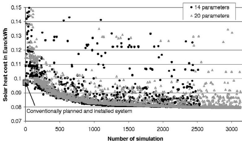
Fig. 3. Optimization of the planning of the solar system in Frankfurt with a Genetic Algorithm. Grey triangular dots represent the optimization with 20 parameters, black dots the optimization with the reduced set of 14 parameters. The results for the solar heat costs during the optimization process are plotted in the figure; the big grey rectangular dot represents the estimated solar heat cost of the installed system.
