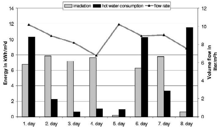
Fig. 5. Optimum flow rates in the collector circuit for the eight investigated days with the corresponding global irradiation in the collector plane and tap water energy both referred to the collector area. It is shown that the flow rate should decrease with an increase of the temperature in the store due to a high global radiation and a low hot water consumption. The values of day five and day eight are not meaningful because of the poor irradiation.
