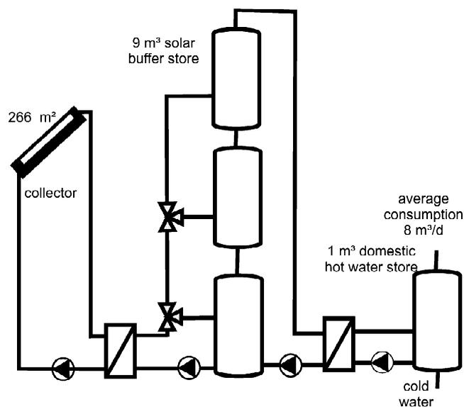
Fig. 2. Design of the SDHW-system of the hospital in Frankfurt/Main. Discharge of the six 1.5 m<sup>3</sup> solar buffer stores takes place depending on the temperature levels in the storage units.
