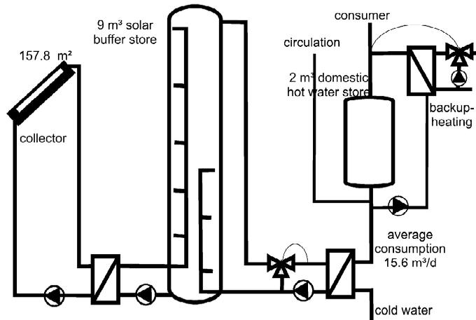
Fig. 1. Design of the SDHW-system of the dormitory in Zwickau. Discharge of the 9 m<sup>3</sup> solar buffer store takes place only during the tapping of hot water.
