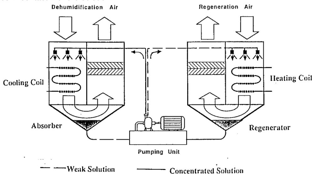
**Figure 8: Schematic of a liquid desiccant system.**
