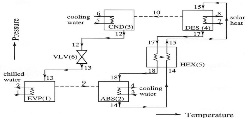
**Figure 2: Single effect solar absorption systems.**
