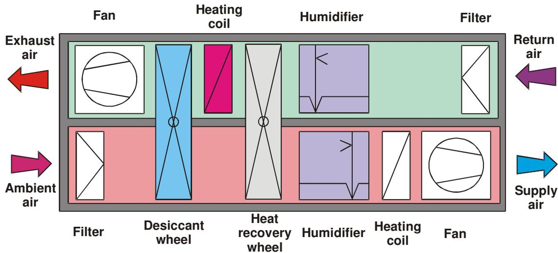
Figure 6: Desiccant heating and cooling unit using an open cycle systems.
