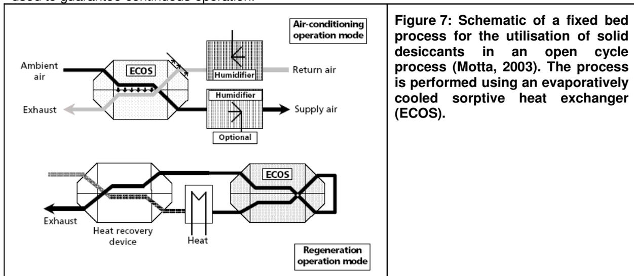
Figure 7: Schematic of a fixed bed process for the utilisation of solid desiccants in an open cycle process (Motta, 2003). The process is performed using an evaporatively cooled sorptive heat exchanger (ECOS).
