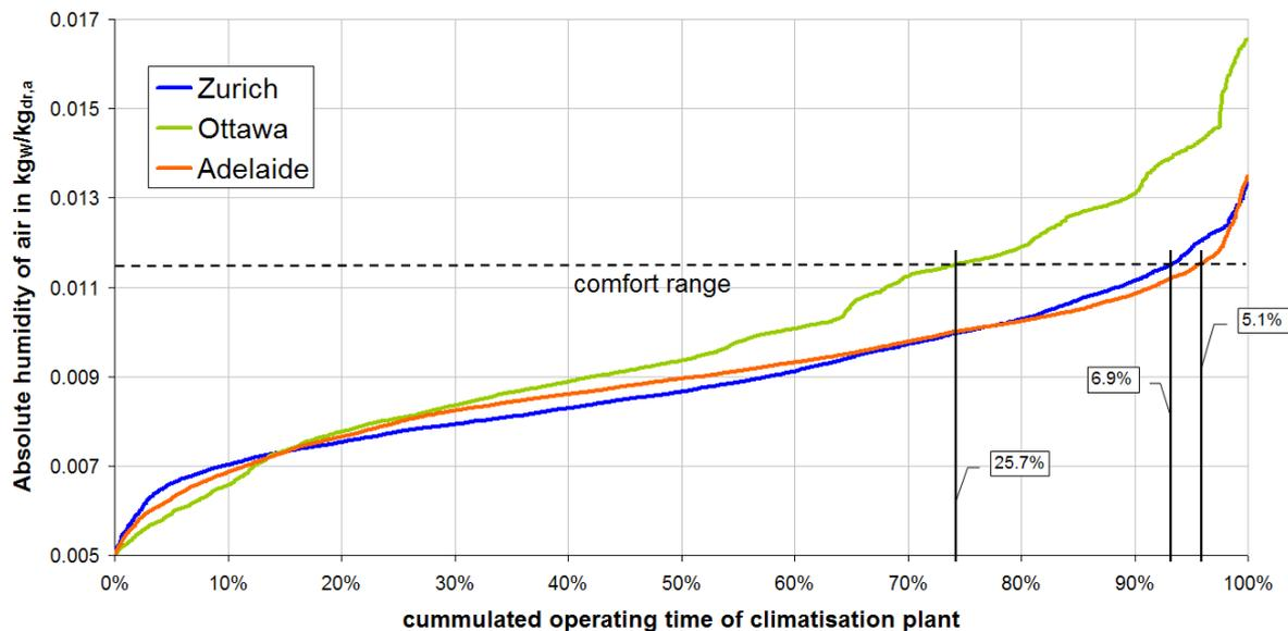
**Figure 3:** Absolute humidity of the room air over the cumulated operation time of the climatisation plant which consists of an indirect evaporational cooler only
