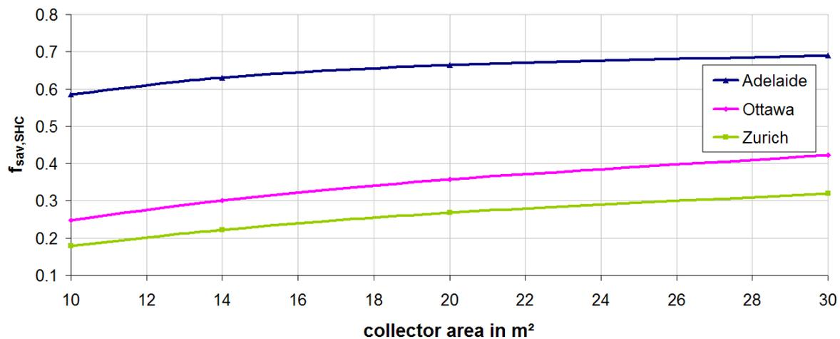
**Figure 2:** Fractional energy savings over the collector area for different climates
