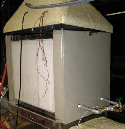
Figure 2: Photograph of the regenerator prototype. Air flows from the bottom to the top in between the plates of the regenerator, desiccant solution wets the cotton layers, introduced by an irrigation system on top of each plate and hot water flows through the channels of the twin walls from the bottom of the front manifold to the top of the rear manifold in a counter/cross flow arrangement.
