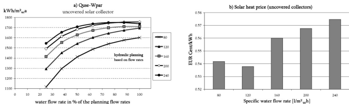
Figure 2: Net solar heat gains without any control at constant flow rates (a) and solar heat price (b) of uncovered collectors used in the described application.
