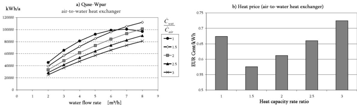
Figure 3: Net heat gains without any control at constant flow rates (a) and heat price (b) of an air-to-water heat exchanger used in the described application.
