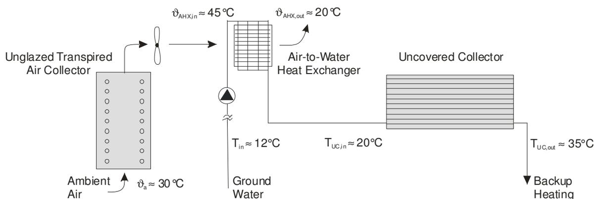
Figure 1: Scheme of the serial connection of a multicomponent solar thermal system with exemplary temperatures [1].
