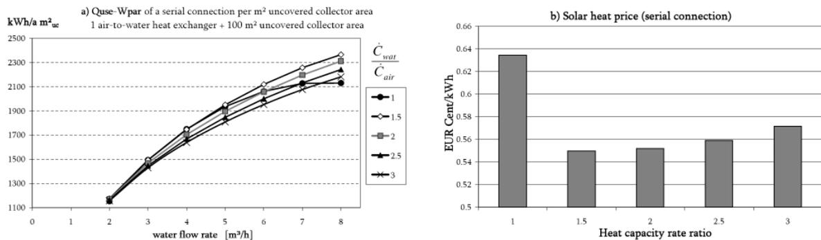
Figure 4: Net heat gains without any control at constant flow rates (a) and solar heat price (b) of a serial connection
