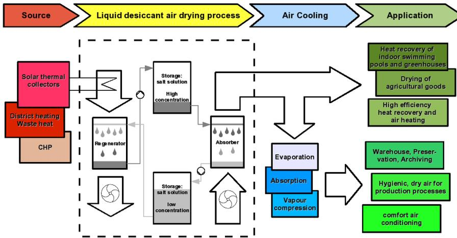
Fig. 1: Liquid desiccant air drying process: from source to application
