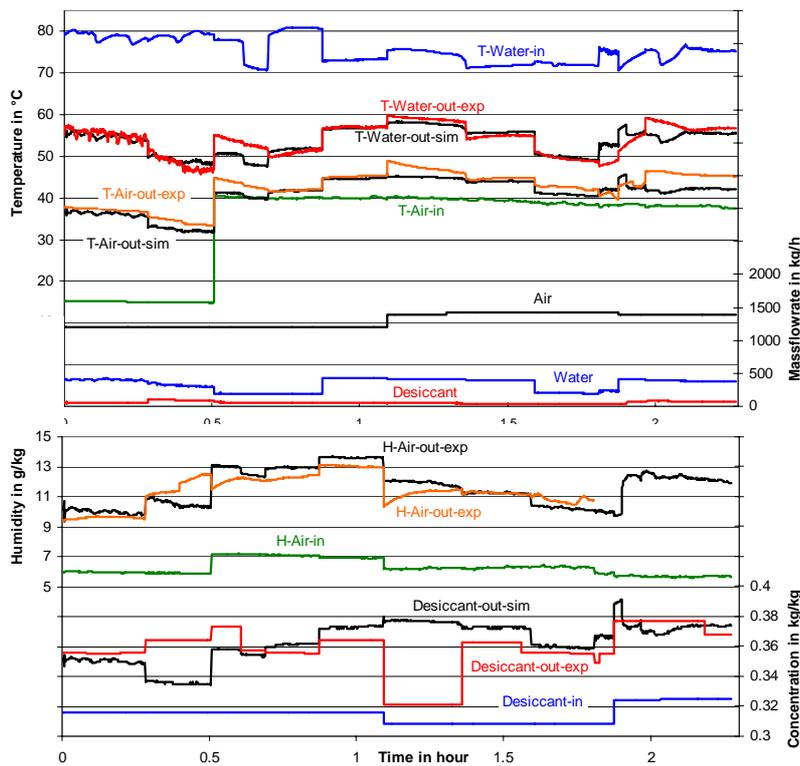
Fig. 3: Simulation and experimental results of the regenerator. The top diagram shows water and air temperatures and the three flow rates, the bottom diagram air humidity and solution mass concentration.
