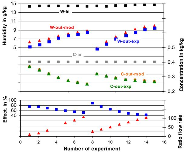
Fig. 2: Comparison of data from the absorber model and 14 sets of experiments gained from Kessling (1998). The top diagram shows air humidity and solution mass concentration (inlet, modeled outlet and experimental outlet conditions), the bottom diagram modeled effectiveness and flow rate ratio between air and solution.
