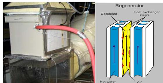
Fig. 1: Photograph of the second regenerator prototype installed in the test rig. The schematic on the right hand side demonstrates the path of air, water and desiccant flows.
