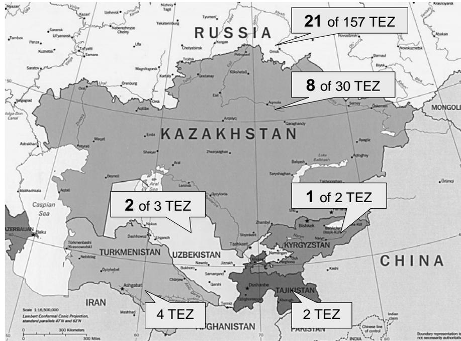
Fig. 5. Geographical distribution of heat and power plants, technically appropriate for a solar preheating
