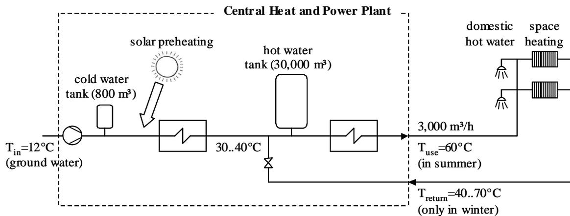
Fig. 1. Simplified hydraulic scheme of a typical open-circuit district heating net in CIS countries (usually without solar preheating), cf. [2]
