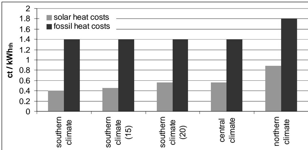
Fig. 6. Solar and conventional heat costs for different locations in the CIS. (15) and (20) represents the water inlet temperature of 15°C and 20°C respectively. Otherwise an inlet temperature of 12°C was assumed.
