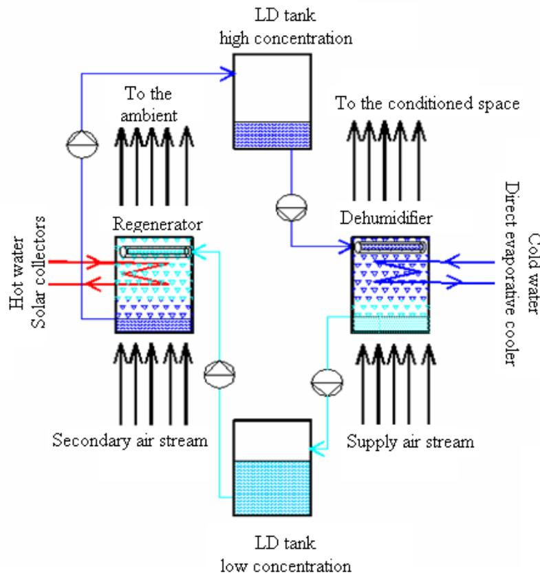
Fig. 1. Schematic of an open-loop liquid desiccant air-conditioning system
