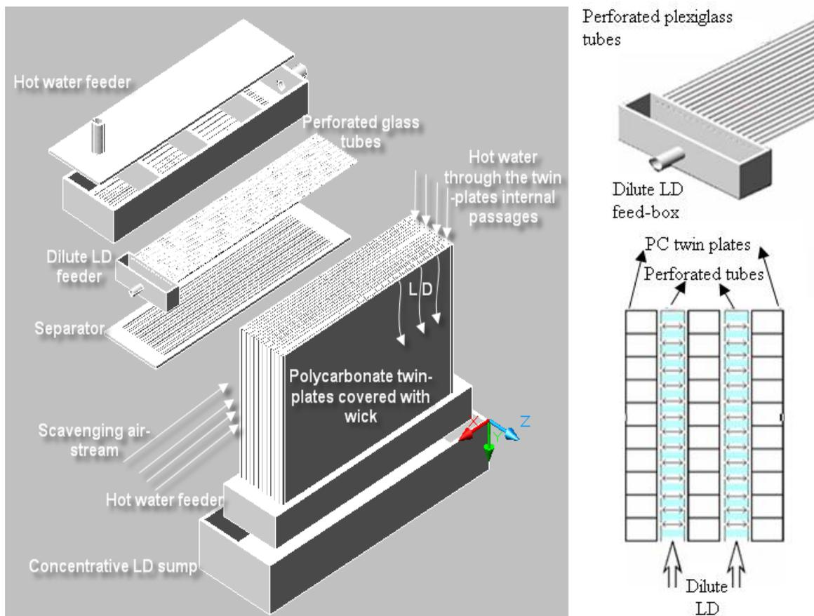
Fig. 2. Exploded view of generator design along with the illustration of flow directions of heating water, LD and air (upper left), an isometric enlargement of the LD distribution system and a top-view of how the glass tubes penetrate the polycarbonate twin-plates (upper right).
