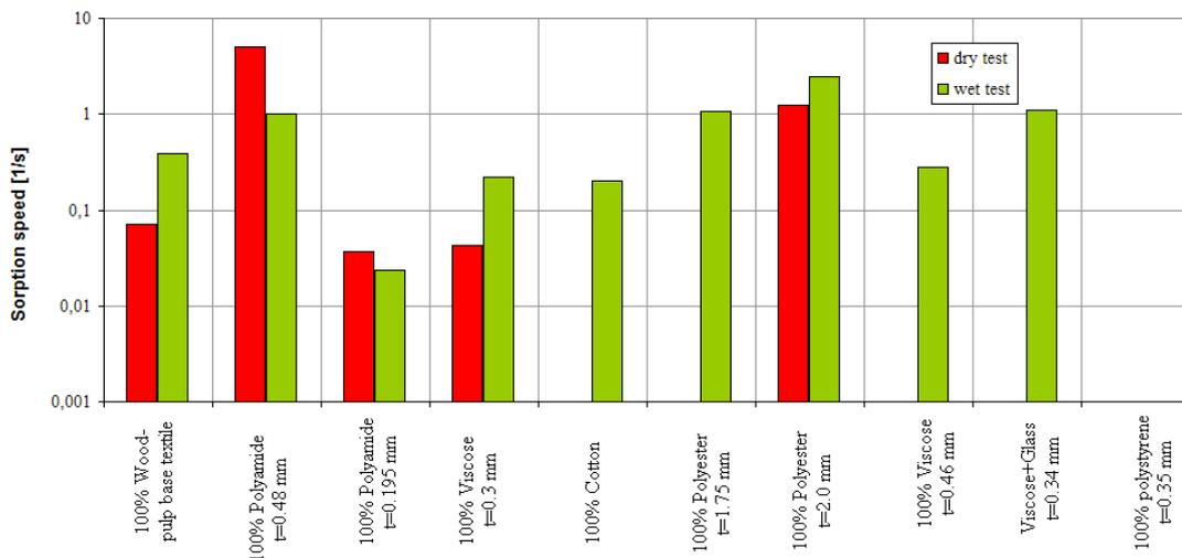
Fig. 6. LiCl adsorption-speed test for different textiles
