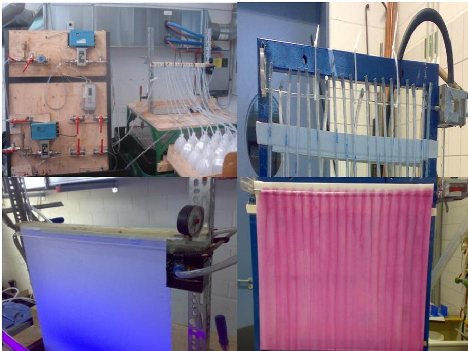
Fig. 3. Experimental setup to determine the optimum size and number of discharge points for the distributor (upper), and to check the LiCl diffusion through the textile (lower).
