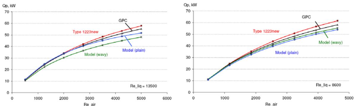
Fig. 4 Heat transfer rate calculated by the model (as plain and wavy fins), Type1223new and GPC for different air flow rates and two geometries (left for HX 1, right for HX 2).
