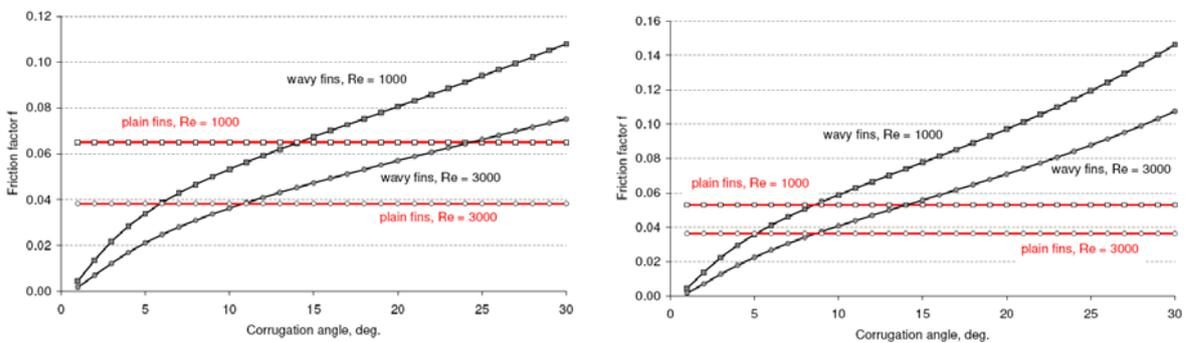
Fig. 2. Influence of the fin corrugation angle on a friction factor  $f$  correlation [12] for two heat exchanger configurations: (a) left HX 2, (b) right HX 3, see Table 1.
