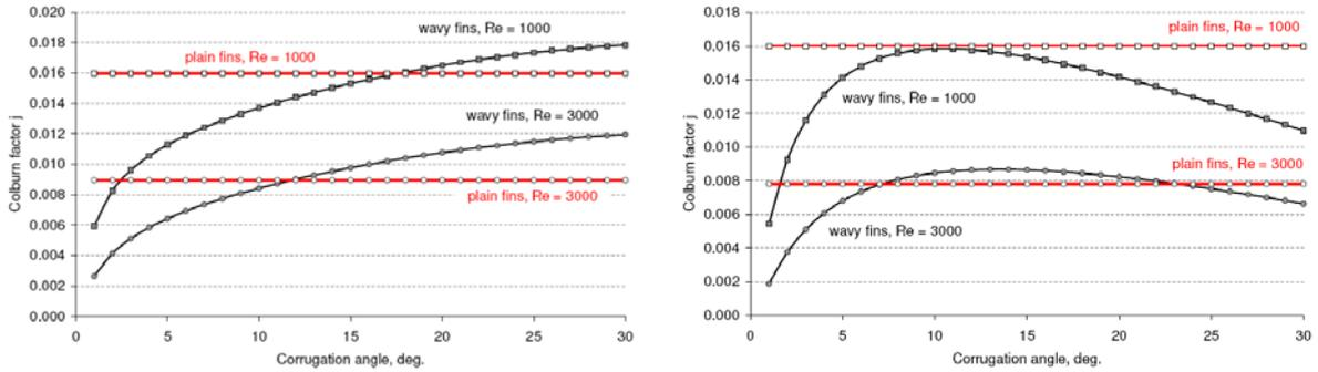
Fig. 1. Influence of the fin corrugation angle on a Colburn factor  $j$  correlation [12] for two heat exchanger configurations: (a) left HX 2, (b) right HX 3, see Table 1. For comparison, values of the Colburn factor for plain fins [10] are also shown.
