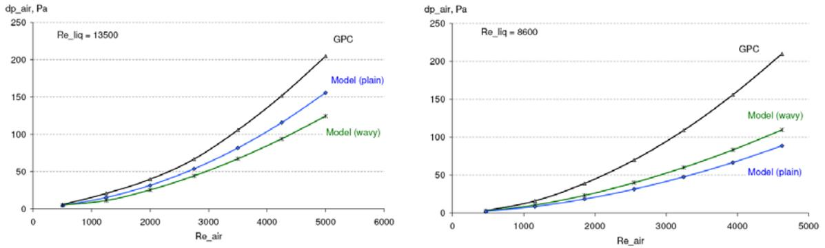
Fig. 5 Airside pressure drop calculated by the model (as plain and wavy fins) and GPC for different air flow rates and two geometries (left for HX 1, right for HX 2).
