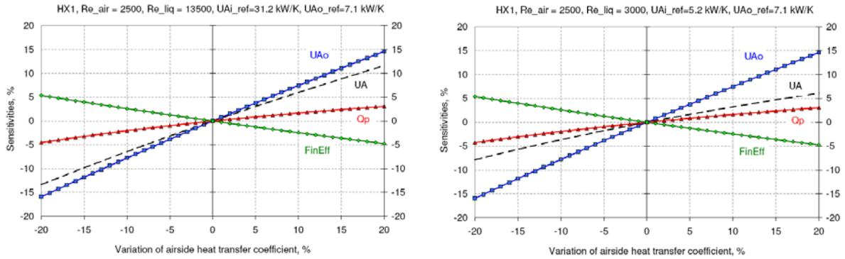
Fig. 3 Heat transfer sensitivities on an airside heat transfer coefficient for geometry HX 1 and two different ratios of UA values on liquid and air sides
