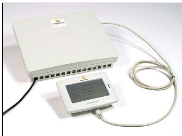
Figure 5. The new developed universal controller, consisting of the hardware unit (top) and the control unit with touchscreen (bottom)
