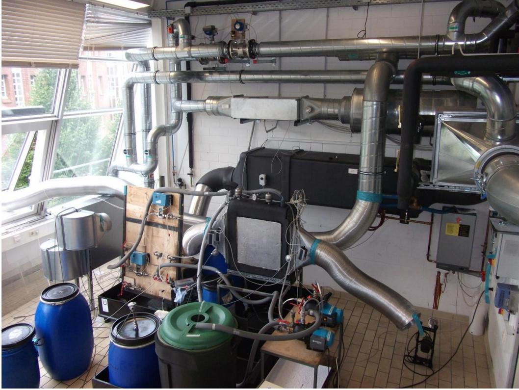
Fig.8. Liquid desiccant dehumidifier test-rig
