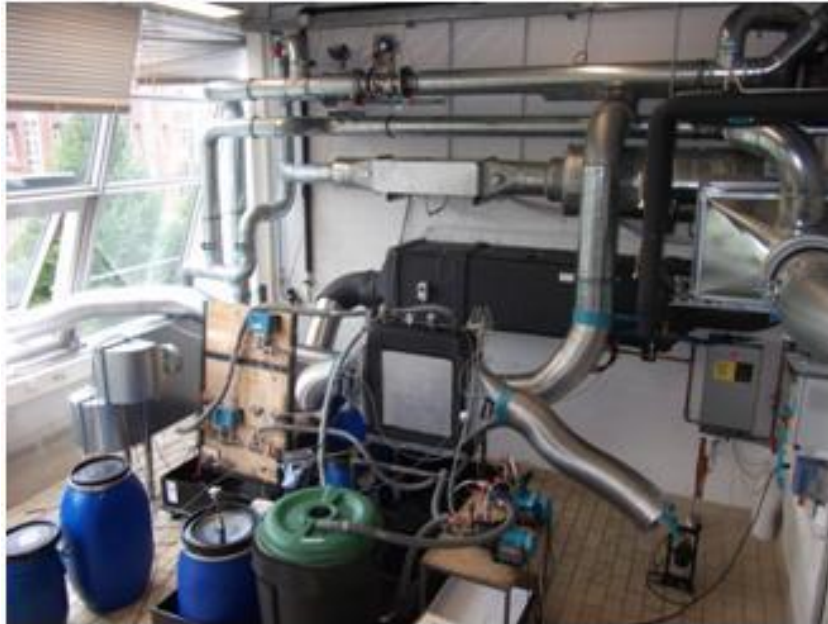
Fig. 2. An overview of the whole liquid desiccant test-rig in the laboratory pilot plant stage
