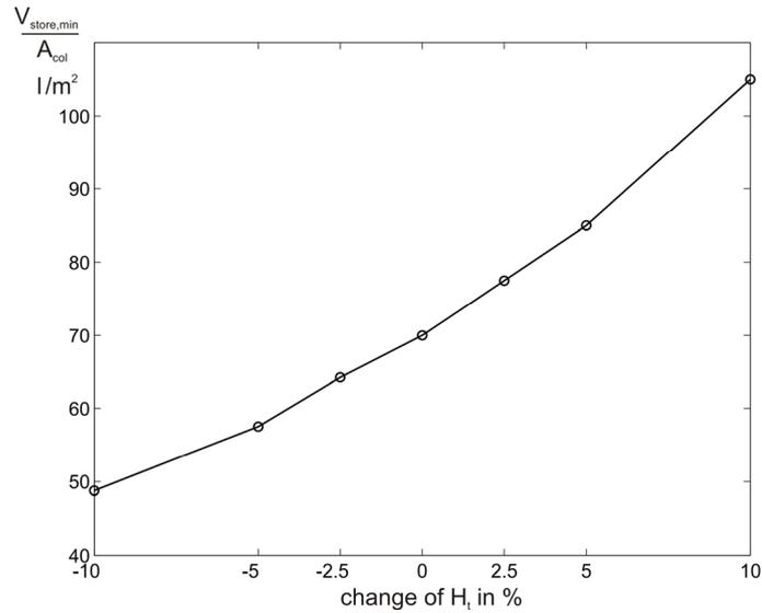
Fig. 4: Influence of global radiation  $H_i$  on minimal specific store volume  $V_{store,min} / A_{col}$ . ( $U_{col} = 3.5 \text{ W/m}^2\text{K}$ ,  $U_{store} = 5 \text{ W/m}^2\text{K}$ )
